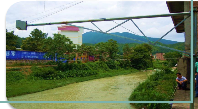
Measuring water flow without touching the water (RQ-30) in Sichuan province 非接触式测流 (RQ-30)，四川
